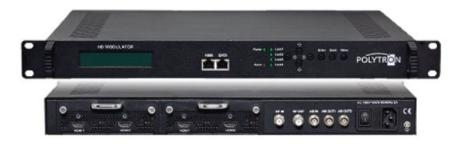
The modulator HDM-8 Q converts four HDMI signals and into two DVB-C (QAM) channels. The video format can be either MPEG2 or MPEG4 standard. The device is wide range useable and can handle HDMI-signals from set-top-boxes, PC/notebooks, cameras, DVD players
