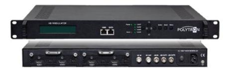
The modulator HDM-8 I converts four HDMI signals and into 8 IPTV channels. The video format can be either MPEG2 or MPEG4 standard. The device is wide range useable and can handle HDMI-signals from set-top-boxes, PC/notebooks, cameras, DVD players
