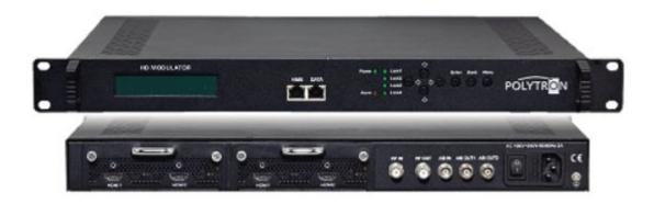
The modulator HDM-4 C converts four HDMI signals and ASI into one DVB-C (QAM) channel. The signal is also available as IP stream and can be fed into IPTV networks. The ASI signal is available for further processing at two outputs. The video format can be either MPEG2 or MPEG4 standard. The device is wide range useable and can handle HDMI-signals from set-top-boxes, PC/notebooks, cameras, DVD players
